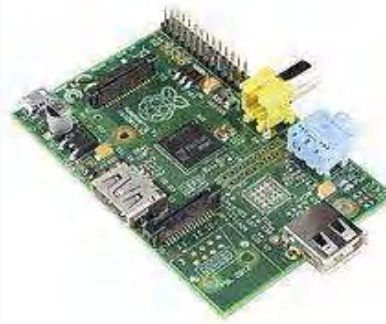
Fig 5.3.3 The early Raspberry Pi 1 Model A, with an HDMI port and a standard RCA composite video port for older displays
