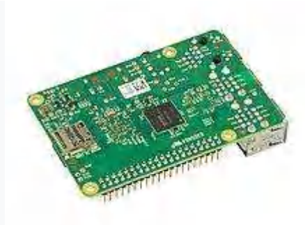
Fig 5.4 Various operating systems for the Raspberry Pi can be installed on a MicroSD, MiniSD or SD card, depending on the board and available adapters; seen here is the
