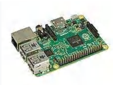
Fig 5.3.2 The Model 2B boards incorporate four USB ports for connecting peripherals.
