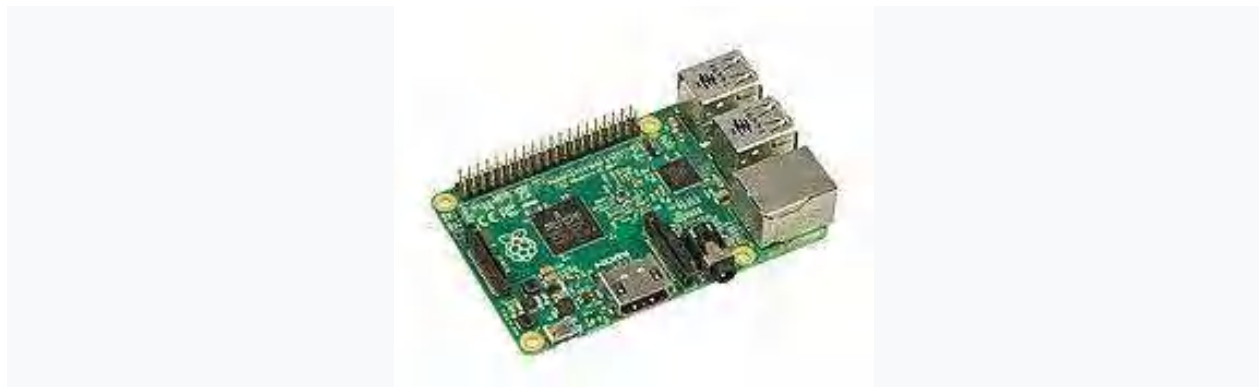
Fig 5.3.1 The Raspberry Pi 2B uses a 32-bit 900 MHz quad -core ARM Cortex-A7 processor.
