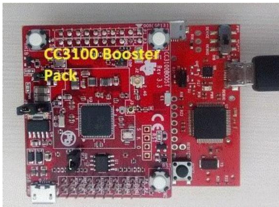
Figure: CC3100 Booster Pack (SimpleLink Wi-Fi) mounted on TIVA Launchpad
