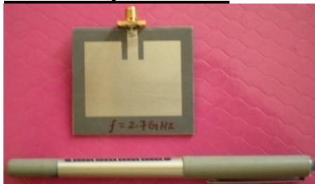
Fig 3.12: Single Microstrip antenna
