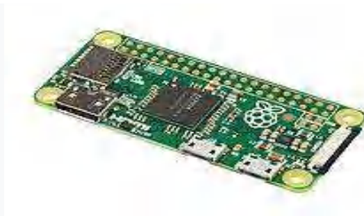
Fig 5.2 The Raspberrv Pi Zero. a US$7 model first introduced in 2015
