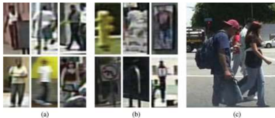
Figure 7: Some hard examples of pedestrian detection from Caltech dataset: (a) small pedestrians, (b) hard negatives, and (c) dense and occluded pedestrians
